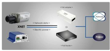
\*) Xpeed IP & Waterproof IP using with High PoE (IEEE 802.3at)
